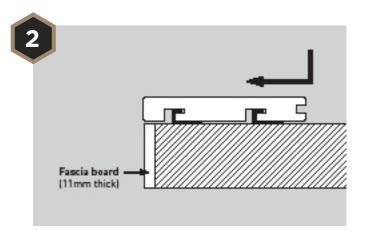
Insert the *HD Deck*<sup>®</sup> *Pro* bullnose deck board over the clips and push it forward. Secure in place with Universal Clips as required.
