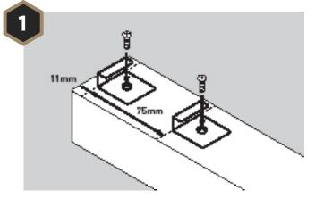
Place two starter clips as shown above, and secure in place with the respective screws. Ensure that the spacing measurements are correct.
