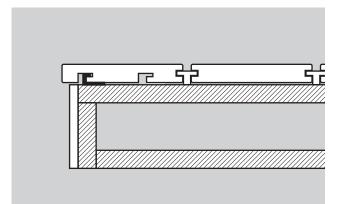
After installing the *HD Deck® Pro* bullnose deck board, as per the above instructions, use the Universal Clip to secure to the rest of the deck. See *Using the New Universal Clip* overleaf.
